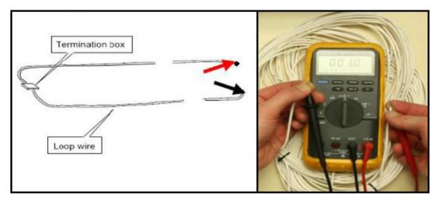
Measure the loop connections. Wait for 5 seconds. Measured value about  $1\Omega$  (Ohm)
