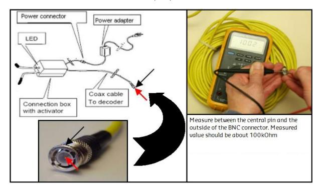
If another value is measured, the connection box with activator is faulty. Replace the part by a new one. Unsolder the detection loop wires from the connection box with activator and measure the detection loop before resoldering the replacement part.
