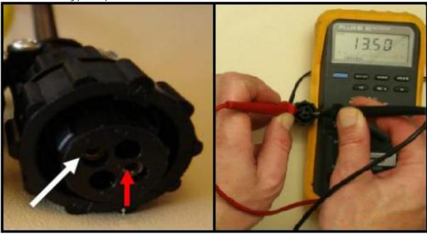
The power supply of the connection box with activator should deliver between 12V DC and 15V DC
