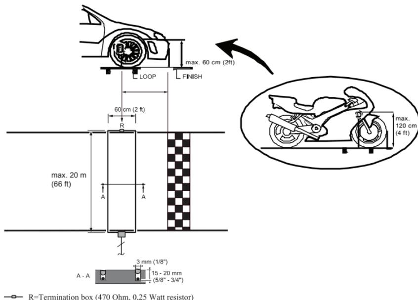
**Figure 2.1 Detection loop installation overview**
