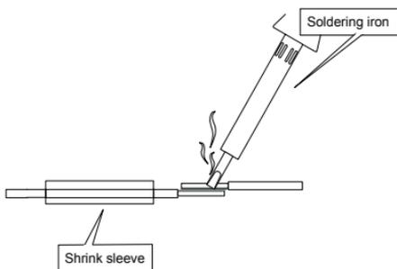
**Figure 2.2 Solder the loop wire end**
