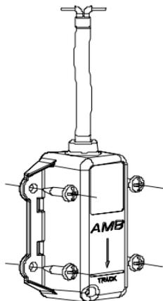
**Figure 3.2 Fastening the Direct Powered transponder**
