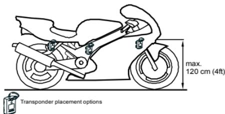
Figure 3.1 Transponder placement
