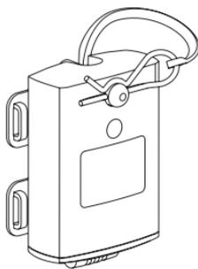
**Figure 3.3 Fastening the transponder in the holder**
